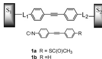
Figure 1. (Top) Schematic of bifunctional, orthogonal self-assembly where L_n refers to a chemical functional group and S_n refers to a substrate to which it preferentially binds. (Bottom) Structures of the molecules used in this study.
